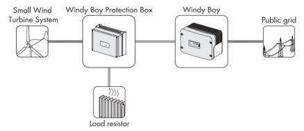
Furthermore, the Windy Boy can be used as an inverter for power conversion units based on permanent magnet generators (hydro power systems, combined heat and power plants, diesel generators, etc.). The manufacturer of the small wind turbine system or the generator must have his plant approved for operation with this Windy Boy (see also the Windy Boy planning guidelines in the download area at www.SMA.de/en).
