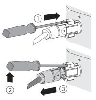
4. Remove the AC connection socket from the inverter.
