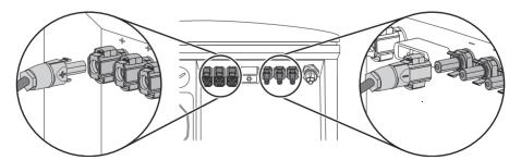
3. Close all unnecessary DC inputs as described in section 5.5.4 "Connecting the Small Wind Turbine System (DC)" (page 32) to seal the inverter.
