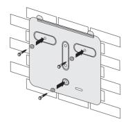
Mount the inverter with the upper fastening plates on the wall mounting bracket so that both plates on the upper edge of the bracket pass through the cutouts on the inverter.
