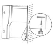
Remove the inverter upwards from the wall mounting bracket.
