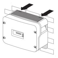
Secure the inverter in position by screwing the supplied M6 contact screw, located on the underside of the enclosure. Use the contact washers provided with the toothing against the enclosure. Tighten the screw with a torque of approx. 5 Nm.
