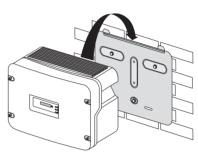
5. **Visual inspection**: The inverter is only correctly mounted when both rear panel mounting plates slightly protrude through the cutouts.
