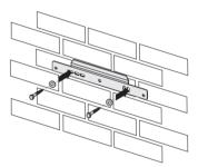
Attach the inverter to the wall mounting bracket using the special opening at the rear of the enclosure.
