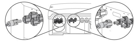
2. To seal the inverter, any unused DC inputs must be closed with DC connectors and sealing plugs.
