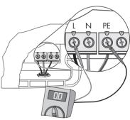
☑ The inverter is open and no voltage is present.
