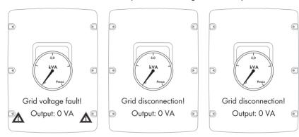
If one of the 3 inverters indicates a device fault and stops feeding in, the other two inverters
