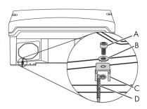
☑ The inverter enclosure is additionally grounded.
