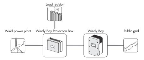
Furthermore, the Windy Boy can be used as an inverter for power conversion units based on permanent magnet generators (hydro power systems, combined heat and power plant, diesel generator, etc.). The manufacturer of the small wind turbine system or generator must have approved his plant for operation with this Windy Boy.
