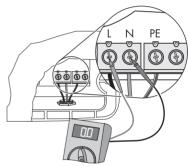
8. Verify the absence of voltage L to PE at the AC terminal with a suitable instrument.
