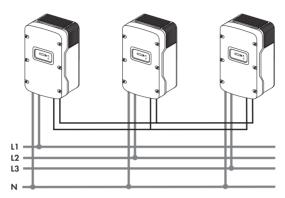
If this electronic circuit is activated, you can specify how the other two inverters should react if there is a device fault in the third inverter or a line voltage fault occurs in its phase.
