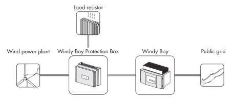
Furthermore, the Windy Boy can be used as an inverter for power conversion units based on the permanent magnet generators (hydro power systems, combined heat and power plants, diesel generator, etc.). The manufacturer of the small wind turbine system or the generators should have his system set up for operation with the Windy Boy (see also the Windy Boy planning guidelines in the download area at www.SMA.de/en).
