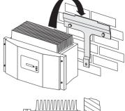
4. Use the provided M6x12 screws to fix the inverter and prevent it from being lifted out of place.
