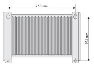
Figure 4: Fixing point distances
