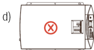
Vertical - this configuration may be used in an environment which is dry and clean only (non-marine)
