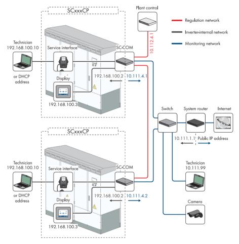
Figure 18: Example of a plant network of 2 inverters with indicator lights
