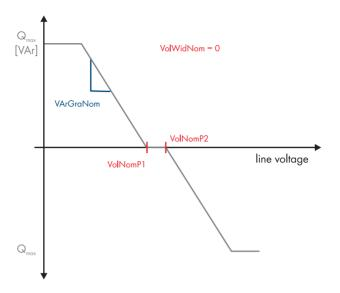
Figure 24: Characteristic curve for reducing reactive power with deadband
