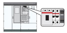
Figure 8: Remote GFDI in the Sunny Central
