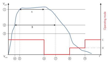
Figure 27: Temporal behaviour of the Sunny Central in the event of grid limits being exceeded
