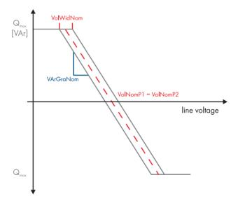
Figure 25: Characteristic curve for reducing reactive power with hysteresis
