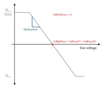
Figure 23: Characteristic curve for reducing reactive power without deadband and without hysteresis
