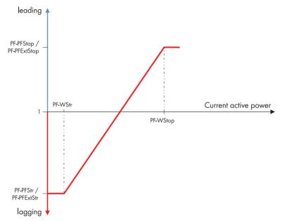
Figure 21: Characteristic curve for reducing reactive power dependent on active power
