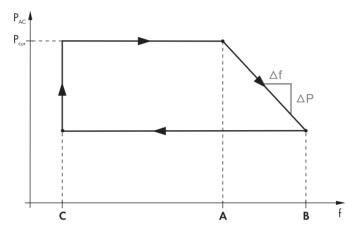
Figure 19: Behaviour of the Sunny Central when the P-HzStr frequency limit is exceeded
