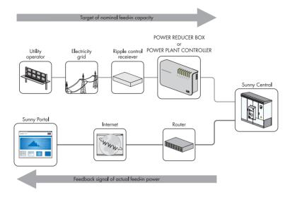
Figure 14: Principle of grid integration
