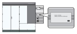
Figure 6: Sunny Central String-Monitor Controller
