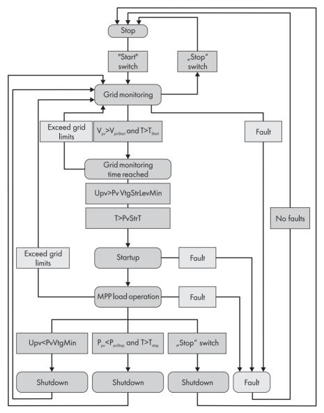
Figure 4: Principle overview of the operating states of the Sunny Central
