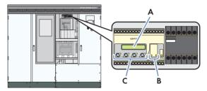
Figure 11: Insulation monitoring device in the Sunny Central
