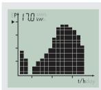
The power and energy of the inverter are displayed as diagrams. The daily power graph is displayed by default.
