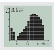
The inverter energy and/or power is shown as a diagram on the display. The daily graph is displayed by default. The right-hand flashing bar of the diagram represents the current hour. If the inverter does not feed any power to the power distribution grid over a longer period of time (e.g. in darkness or if the PV modules are covered with snow), a gap is inserted into the chart. The column for the current hour is updated automatically every five seconds.
